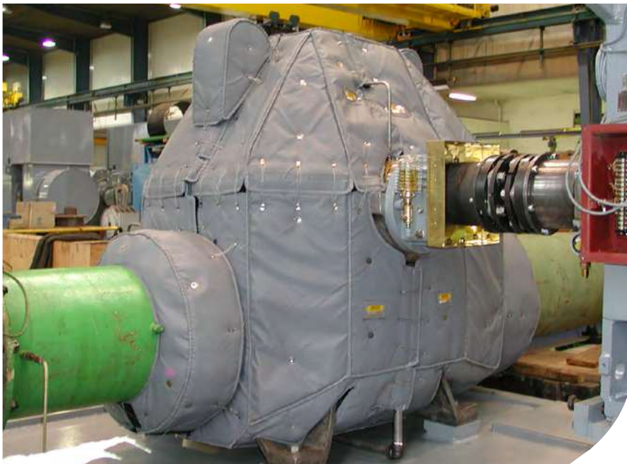
16"x18" CENTRIFUGAL PUMP Design: LT450A-TT – 1.5" thick 6.0 dBA Reduction
