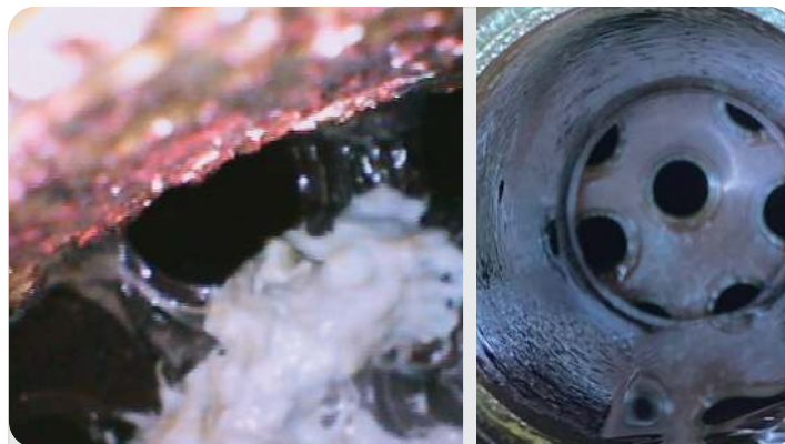
Buildup on heat exchanger tubes after 2 months use, and no buildup after continued use of nanobubble generator.
