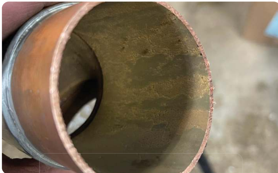
Nanobubbles starting to remove scale on a sample of pipe from Memorial Healthcare’s domestic hot water system.
